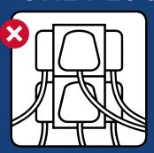
Don't overload your plug sockets. Appliances such as washing machines should have a single plug to themselves as they are high powered.
